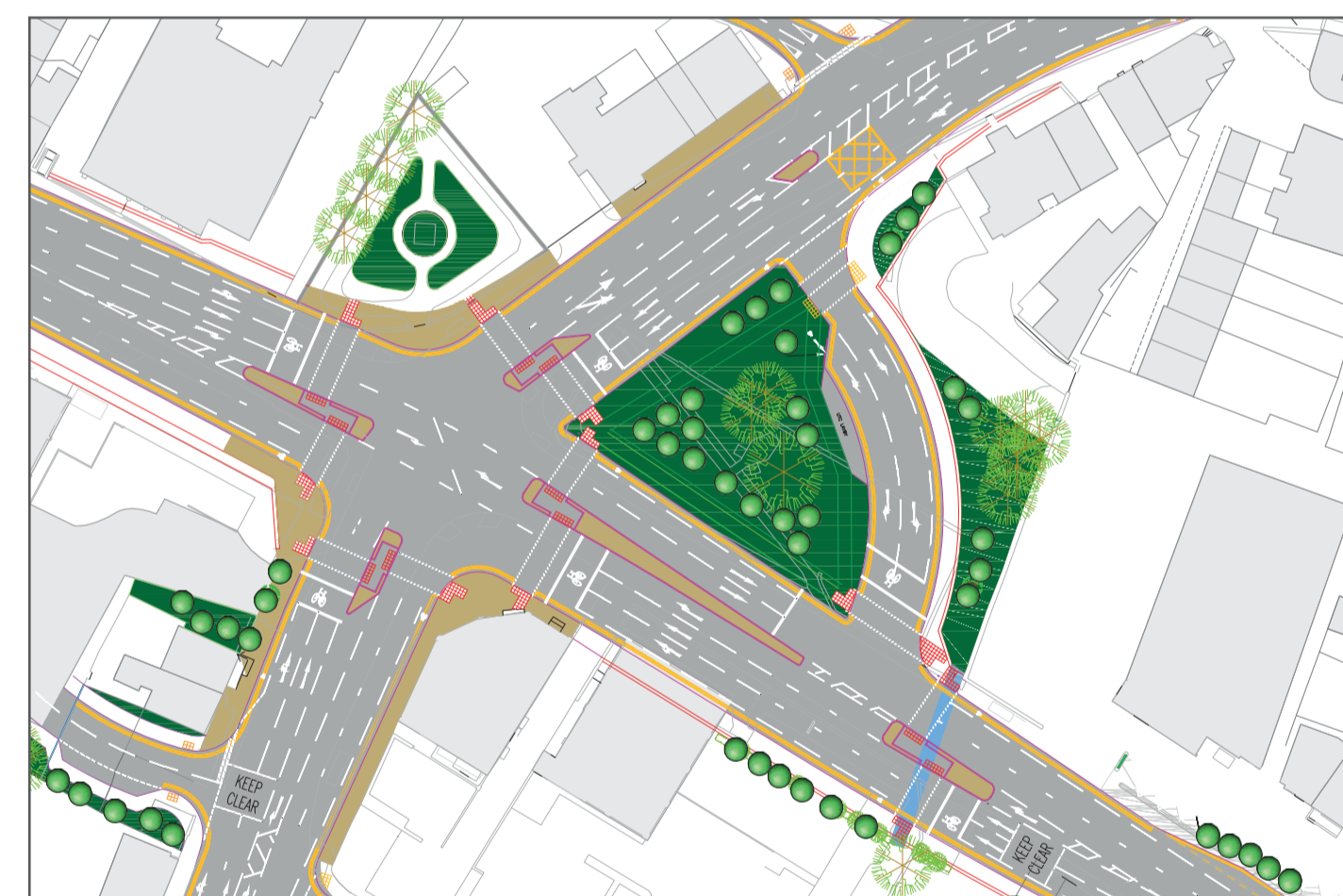
An indicative plan showing the proposed section of road that will be installed allowing a left and a right turn from Harrogate Road onto New Line.
